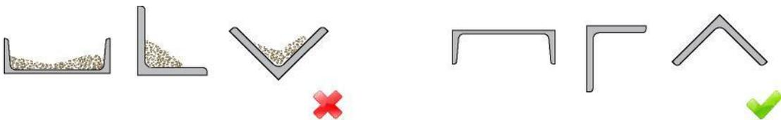
Figure 3a - Prevent water and dirt from accumulating
