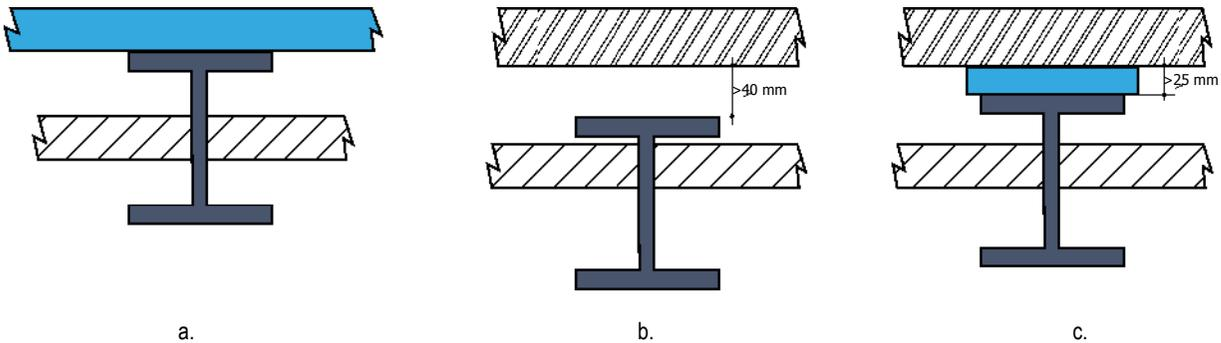
Figure 1: the steel structure is protected against water from the outside (horizontal cross-section)
