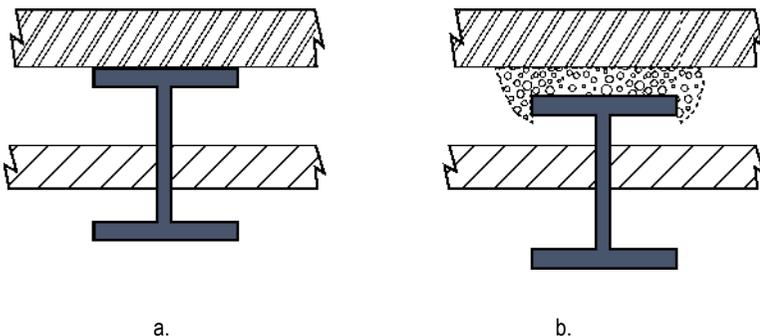
Figure 2: the steel structure is exposed to water from the outside (horizontal cross-section)
