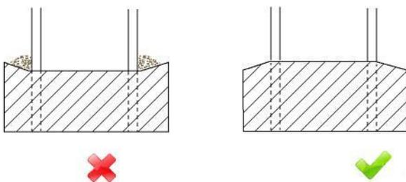
Figure 3b - Prevent water from remaining at the foot of a column
