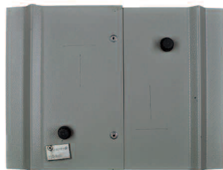
Figure 13. A Colorcoat HPS200 Ultra® test panel after more than 2 years exposure at Brest
