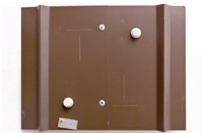
Figure 16. Colorcoat HPS200® with Galvalloy® metallic coating – 6 years exposure at coastal weathering site at Rye, England.
