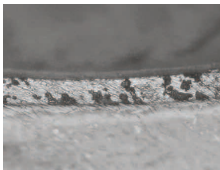
Figure 9. Galvalloy® microstructure after corrosion
