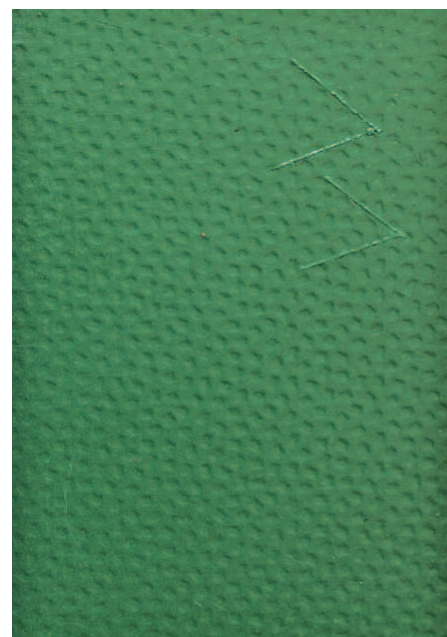
Figure 29. Heritage Green standard leathergrain and Colorcoat HPS200 Ultra® after 2000 total hours in UVB test
