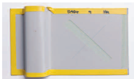
Figure 21. Test panel after humidity 1000 hours
