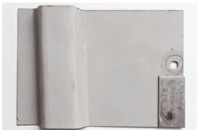
Figure 17. Colorcoat HPS200® with Galvalloy® metallic coating – 13 years exposure at coastal weathering site at Rye, England.
