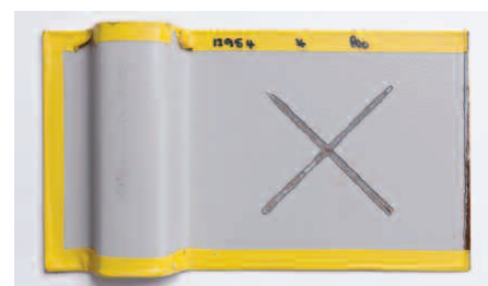
Figure 22. Test panel after Watersoak 1000 hours
