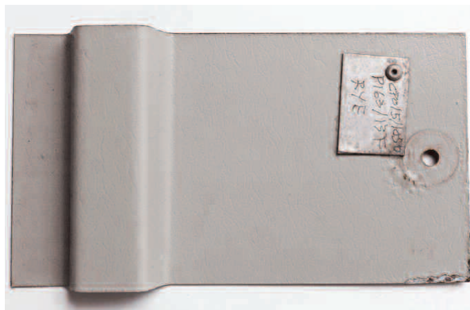
Figure 18. Colorcoat HP200® 18 years exposure at coastal weathering site at Rye, England.
