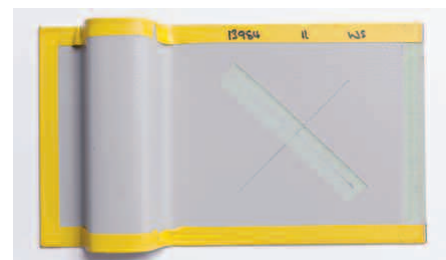
Figure 22. Test panel after Watersoak 1000 hours
