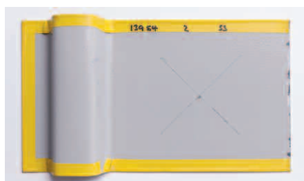
Figure 21. Test panel after humidity 1000 hours
